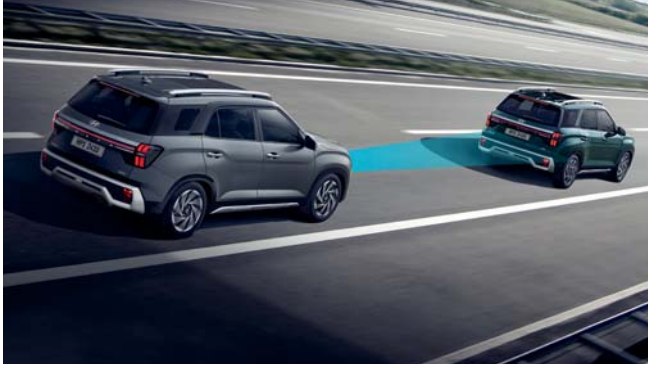
Smart Cruise Control with Stop & Go (SCC with S&G) Smart Cruise Control (SCC) helps maintain distance from the front vehicle and drive at a speed set by the driver. Automatically stops when the front vehicle stops and automatically starts when the front vehicle departs within a short time.
