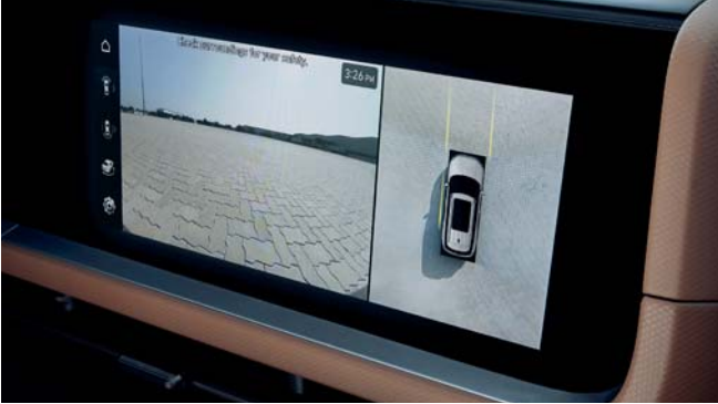
Surround View Monitor (SVM) Surround View Monitor (SVM) displays images of the situation around the vehicle in various views for safe parking.
