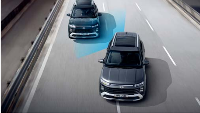
Blind-Spot Collision-Avoidance Assist (BCA) Ind-Spot Collision-Avoidance Assist (BCA) warns you if there is a risk of collision with a rear side vehicle in the blind-spot while changing lanes. When forward exiting a parallel-parking spot, if there is a risk of collision with a vehicle approaching from behind, it automatically assists with emergency braking.
