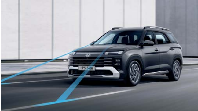
Lane Keeping Assist (LKA) If driving above a certain speed and the driver leaves a lane without the turn signal switch being operated, it provides a warning. When a lane departure is detected, it automatically assists with steering to help prevent leaving the lane.
